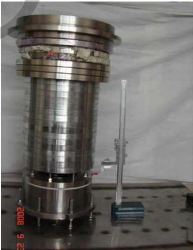
图 5 拉力测量试验装置 Fig. 5 Test device of the pulling force measurement
